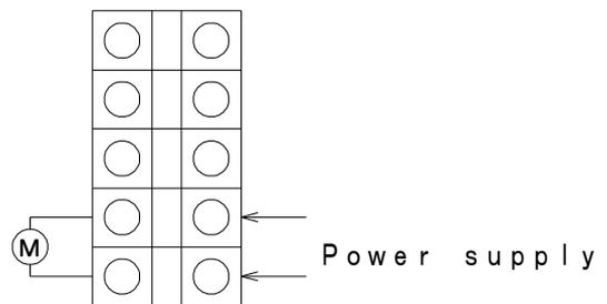
• Terminal connection (With oil level switch)
